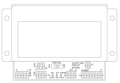
The control module includes three diagnostic LED's for ease of servicing. These LED's are located on the center of the board, near the edge. They are labeled "IPX FAULT", "IPX OK, and "WIRING FAULT".
