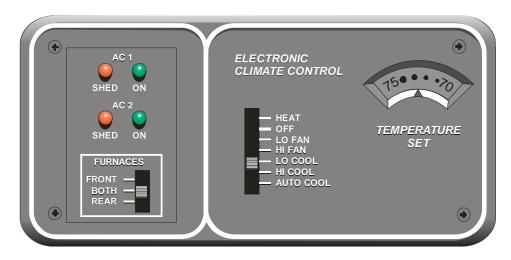
There is a single function switch that controls the functions of the two air conditioner (A/C1) and (A/C2) systems. The potentiometer allows the user to select a desired temperature for the system in the range of 50 to 90 degrees Fahrenheit. Moving the controls down lowers the set point temperature. The seven-position function switch is used to select the furnace's and air conditioners' operating modes.
