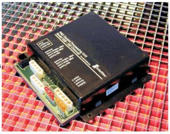
The approximate module dimensions are 6.375" X 6.250" X 1.875" (16.2mm X 15.9mm X 4.8mm). The module should be installed in a protected environment inside of the vehicle.
