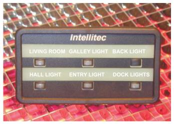
Switch Legends printed on paper with computer printer. Paper placed under overlay w/clear windows.
