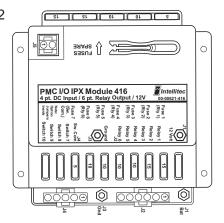
Four inputs labeled Switch 1 - 4 can be individually set for either positive (high-side) switched to the battery, or negative (low-side) switched to ground. Setting a jumper to short pins AB selects positive switch. Setting a jumper to short pins BC selects negative switch.
