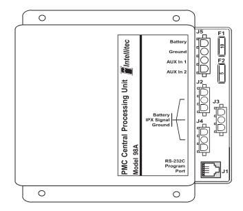
The CPU can communicate with up to 16 modules. Each module can have a combination of up to 10 inputs or outputs, with a single CPU controlling up to 160 inputs/outputs. If your system requires more than 160 I/O points, CPU 00-00800-021 can be used.
