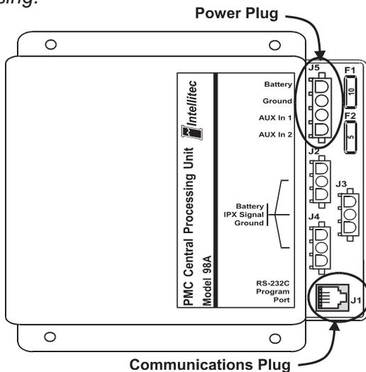
Connect the computer to the CPU Module using the RJ11 telephone cable and the hardware adapter key. Plug the adapter into the serial port of the computer. Plug the RJ11 cable into the adapter and then into the module.
